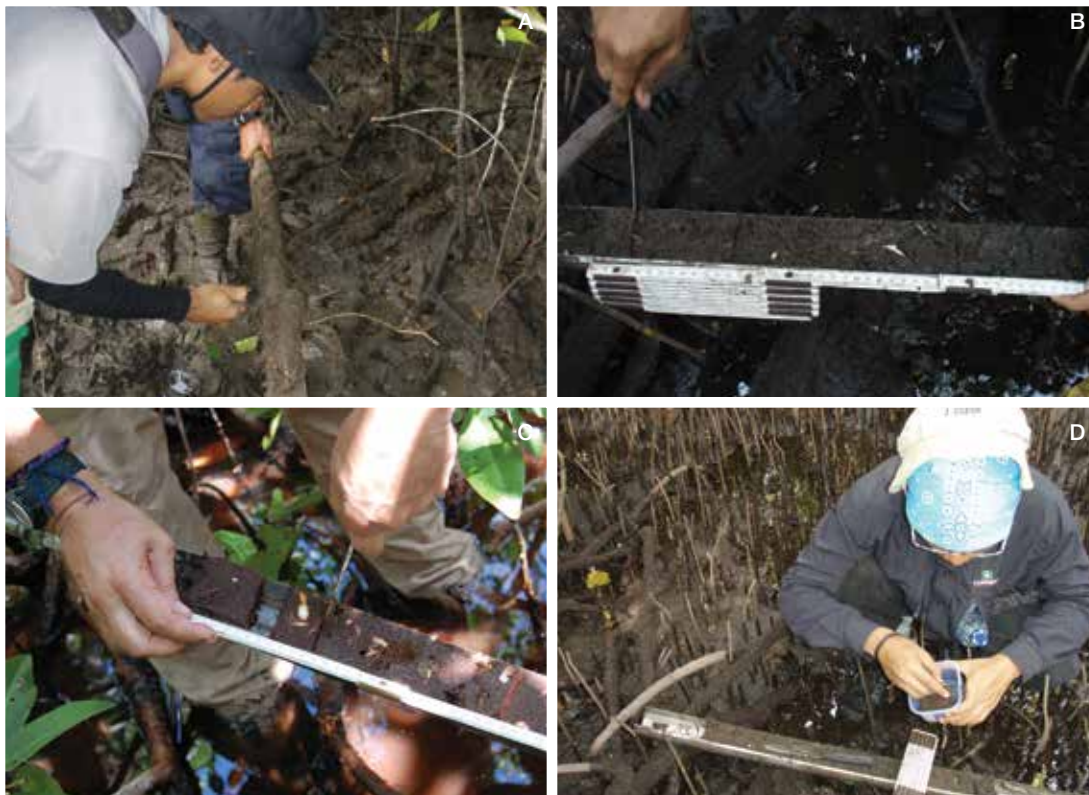
Figure 3.15 Collection of soil samples from open-face auger. (A) Cutting soil away from auger face, (B) Measuring and marking the depth intervals, (C) Cutting a sample, (D) Removal of sample from auger in numbered container (© Boone Kauffman, OSU)
