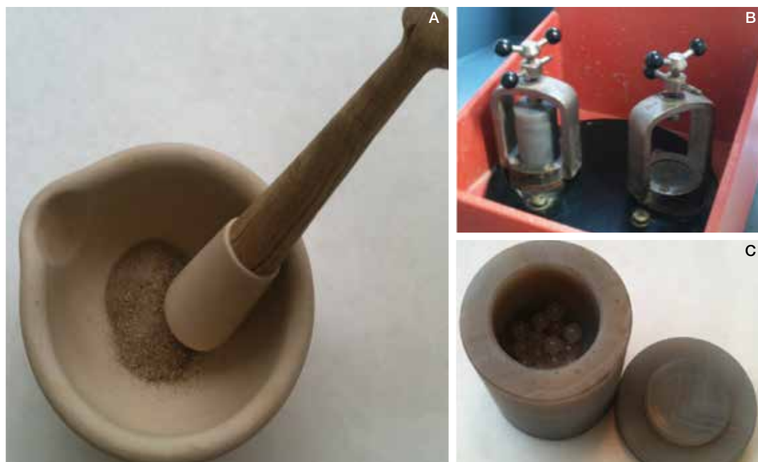
Figure 3.21 Grinding and homogenization of a soil sample. (A) Mortar and pestle, (B) Agate pot in commercially available mill, (C) Agate pot with beads to help pulverize and homogenize the soil sample. (© Hilary Kennedy, UWB)
