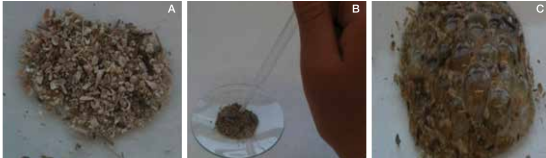
Figure 3.24 Testing for carbonate. (A) Subsample in a watch glass prior to acidification, (B) pipetting a few drops of weak HCl, (C) subsample effervescing. (© Hilary Kennedy, UWV)
