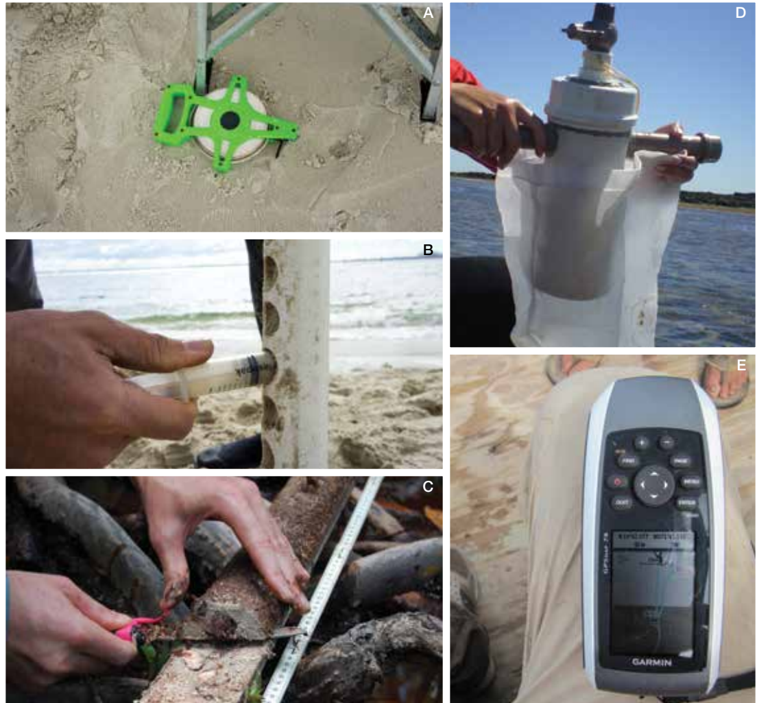
Figure 3.3 Equipment typically needed for field collections of soil carbon. (A) Measuring tape for measuring depth along the soil core (© Sarah Hoyt, CI), (B) Syringe used to subsample core (© Sarah Hoyt, CI), (C) Knife used for subsampling (© Boone Kauffman, OSU), (D) Core & sample bag (© Krishna Barros, UFC), and (E) GPS to mark coring position (© Boone Kauffman, OSU)
